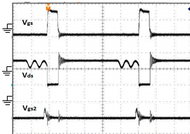
Figure 9. The valley-switching waveforms V_{gs} , V_{ds} , and V_{gs2} at a light load when the input DC voltage is 380 V_{dc} . ( V_{gs} : 10 V/div, V_{ds} : 10 V/div, V_{GS2} : 10 V/div, time: 2 \mu s/div).
